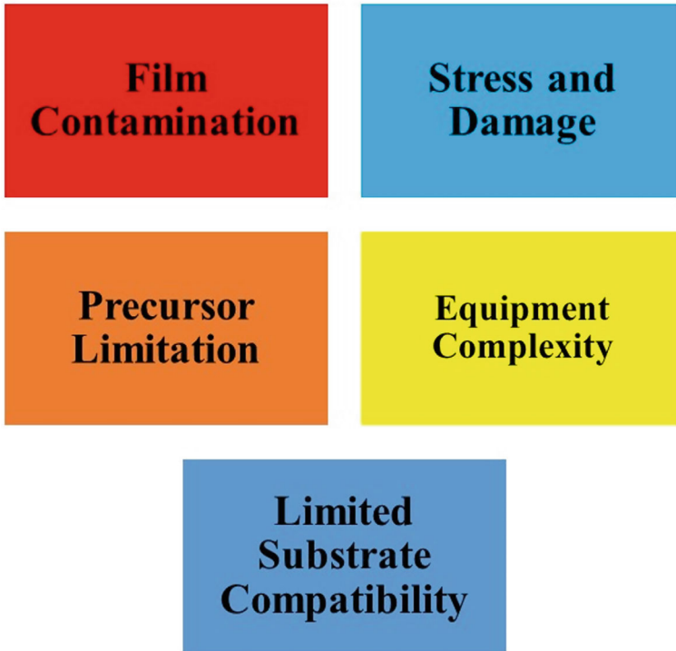
Fig. 3.8 Some disadvantages of low-pressure CVD
